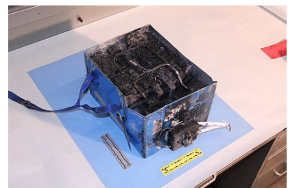
Japan Airlines Boeing 787 lithium cobalt oxide battery that caught fire in 2013
