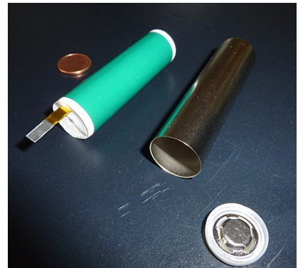
Cylindrical Panasonic 18650 lithium-ion battery cell before closing.
