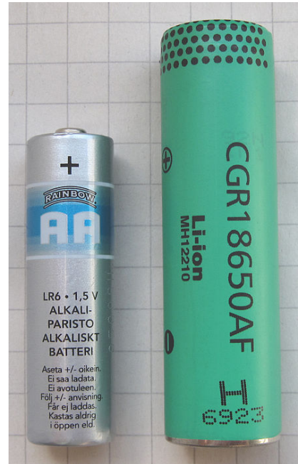
An 18650 size lithium ion battery, with an alkaline AA for scale. 18650 are used for example in notebooks or Tesla Model S
